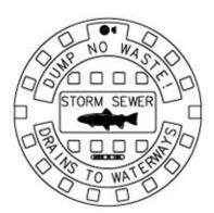
Marking requirements also apply to manholes placed to access public or private catch basins/inlet boxes.
