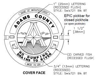
All <u>privately</u> owned storm sewer manhole covers shall be permanently imprinted with the image of a fish and must incorporate the following information (or equivalent):
