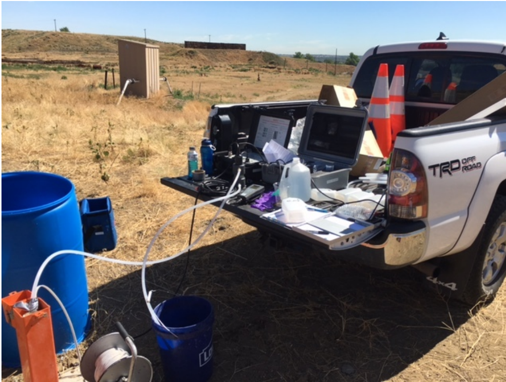
Developing groundwater monitoring well AC-MW1
