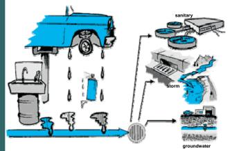
Managers need to understand that interior drains discharge into the sanitary sewer, but outdoor drains discharge directly into the environment.
