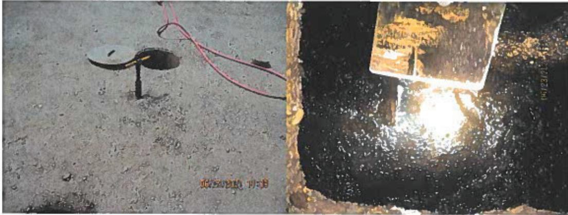
Probe able to pass through top of secondary tank
